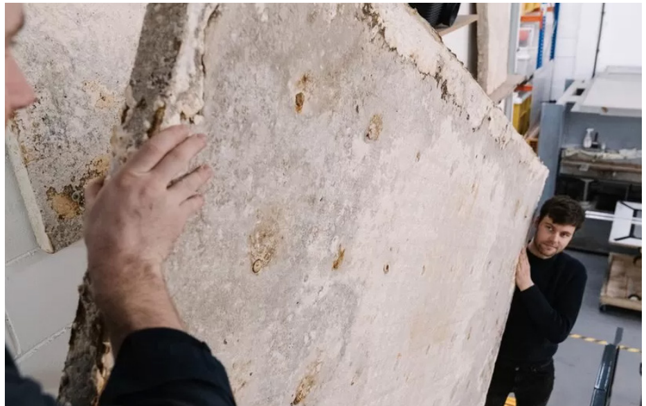
Building blocks: Mycelium can be used to make wall insulation to keep houses warm.
